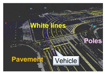
3. Obstacle detection by matching with sensor data
