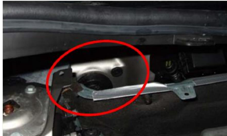
Figure D.1 — Location of ground installation point
