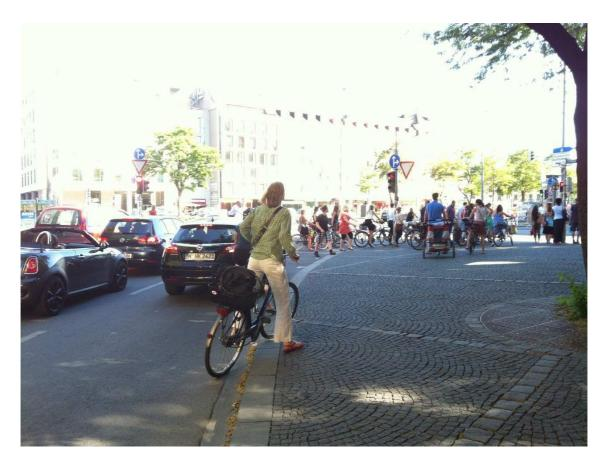
Figure 2: Cyclists going southward do not have space to wait next to cars on the traffic light and therefore change to the sidewalk, which is highly frequented by pedestrians and other cyclists coming from the east.
