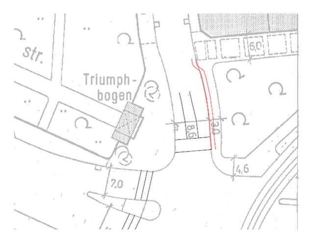
Figure 13: Possible implementation of a contra-flow lane on Sophienstrasse which would not reduce the number of lanes for cars
