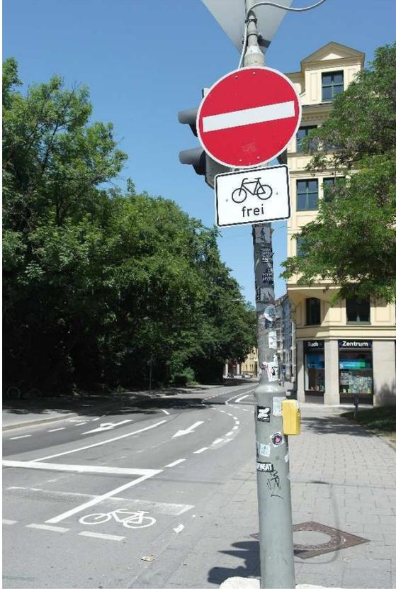
*Figure 18: The sign allows cyclists to enter Sophienstrasse in contra-flow direction*
