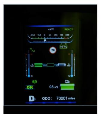
Intelligent Speed Assistance keeps bus speeds to the posted speed limit (through acceleration retardation), thereby preventing buses from exceeding the limit.
