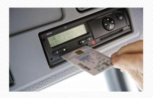
The digital tachograph was developed 1997-2002 and launched (after a 2 years delay) in 2006 to facilitate and enhance drivers hours controls for companies, drivers and enforcers
