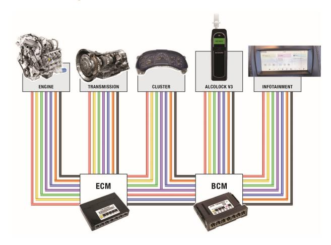
The new digital interface as per EN50436-4 allows quick and safe installation of alcohol interlocks and defines communication protocol over CAN or LIN networks
