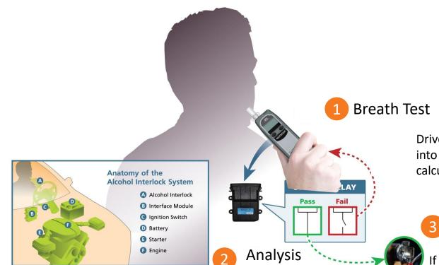
The interface module receives alcohol measurement and decides whether to allow the vehicle to start. Driver provides breath sample into alcohol interlock which calculates breath alcohol level.
