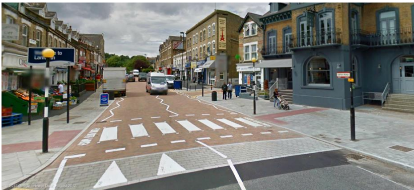
Raised tables reduce average speeds by 17-18 per cent
