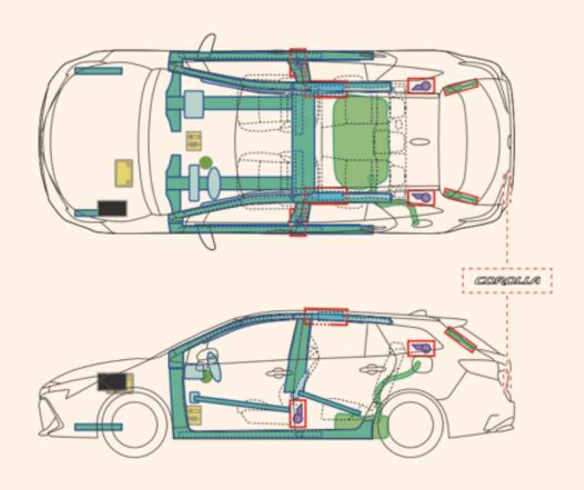
Detail from a rescue sheet identifying vehicle structure and key components<sup>7</sup>
