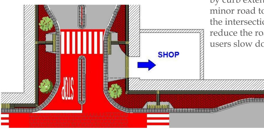
We increased the sidewalk width by curb extension, especially in the minor road to prevent parking in the intersection's proximity and to reduce the road width to make the users slow down.
