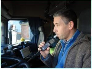
There is a link between the alcohol interloc and the on board computer. In case of a positive test, an alarm is generated. The new European regulation of 0,2‰ is implemented
